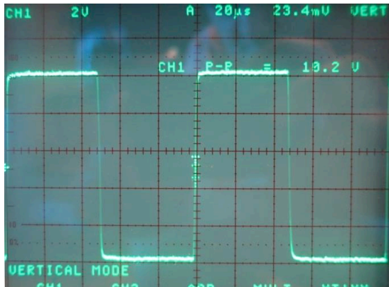
Figure 14: 10 kHz square wave with no reconstruction filter
