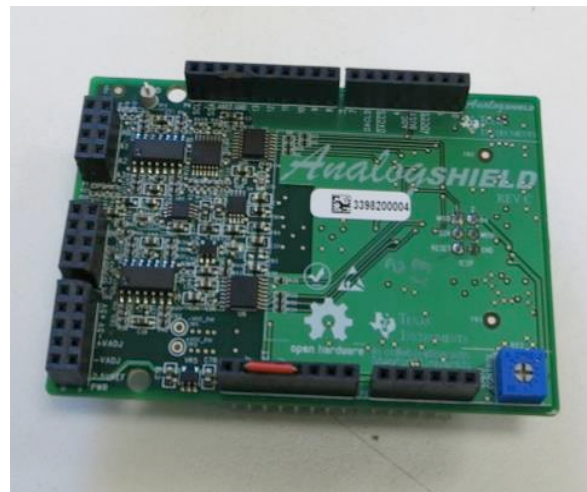
Figure 2: Prototype Analog Shield, with breadboard not attached.
