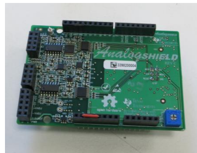
Figure 2: Analog Shield, showing space for prototyping breadboard.
