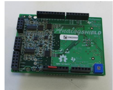
Figure 3: Analog Shield without breadboard.
