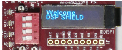
Figure 2.17: DSP Shield OLED display, user DIP switches, and user LEDs.
